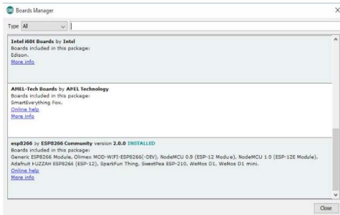
Figure 9: ESP 8266 board installation in Arduino
